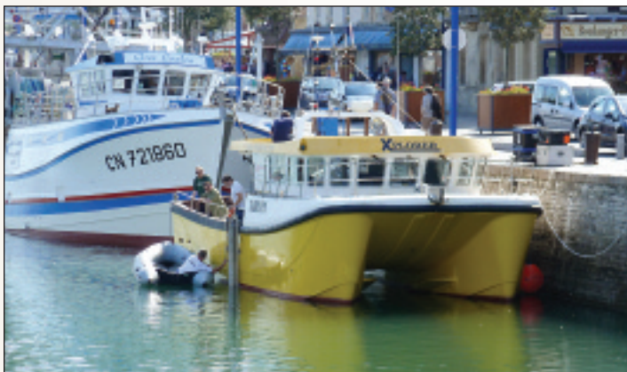
The survey boat ‘Xplorer’ alongside the pier in Port en Bessin. The multi beam echo sounder, now attached to the boat and in its deployed position, is checked for the accuracy of the fit.
